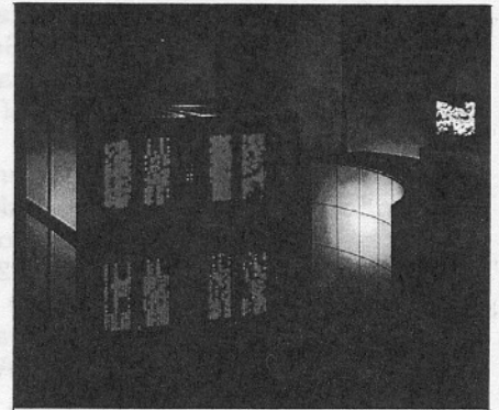
The CM-2 massively parallel supercomputer uses thousands of processors to achieve speeds in tens of gigalops, coupled with gigabytes of main memory and very fast I/O subsystems.
