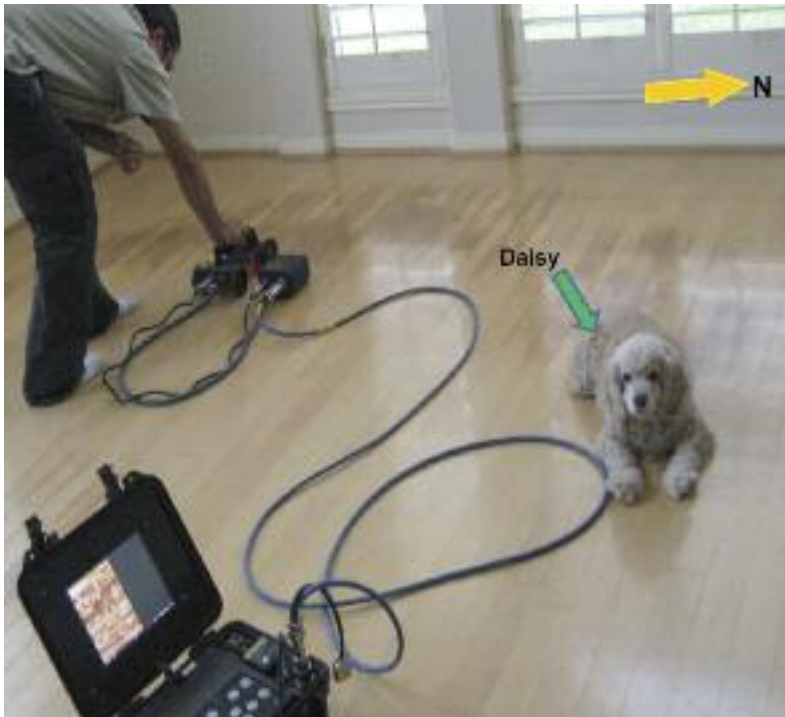
Figure 3. Picture showing the 1500 MHz GPR survey in the living room. The GPR data was collected at every 6 inch.
