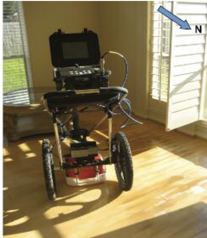
Figure 4. Picture showing the 400 MHz GPR survey in the living room. The GPR data was collected at every one foot.
