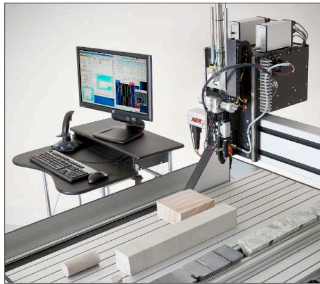
Figure 1. AutoScan – robotically-controlled gantry system for physical property measurements of several different types of core.
